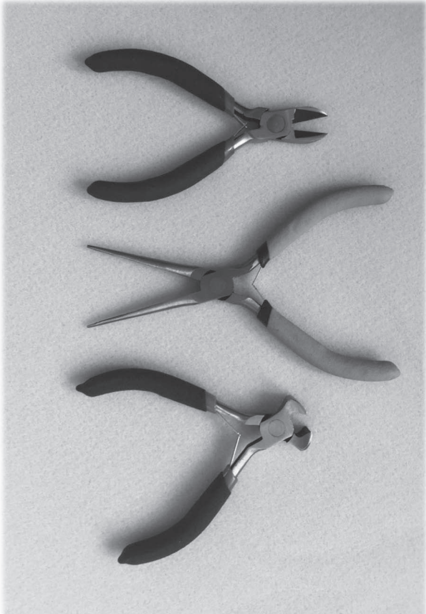
15. Jewellery pliers: top - side cutter middle - long/needle nosed bottom - snub nosed
