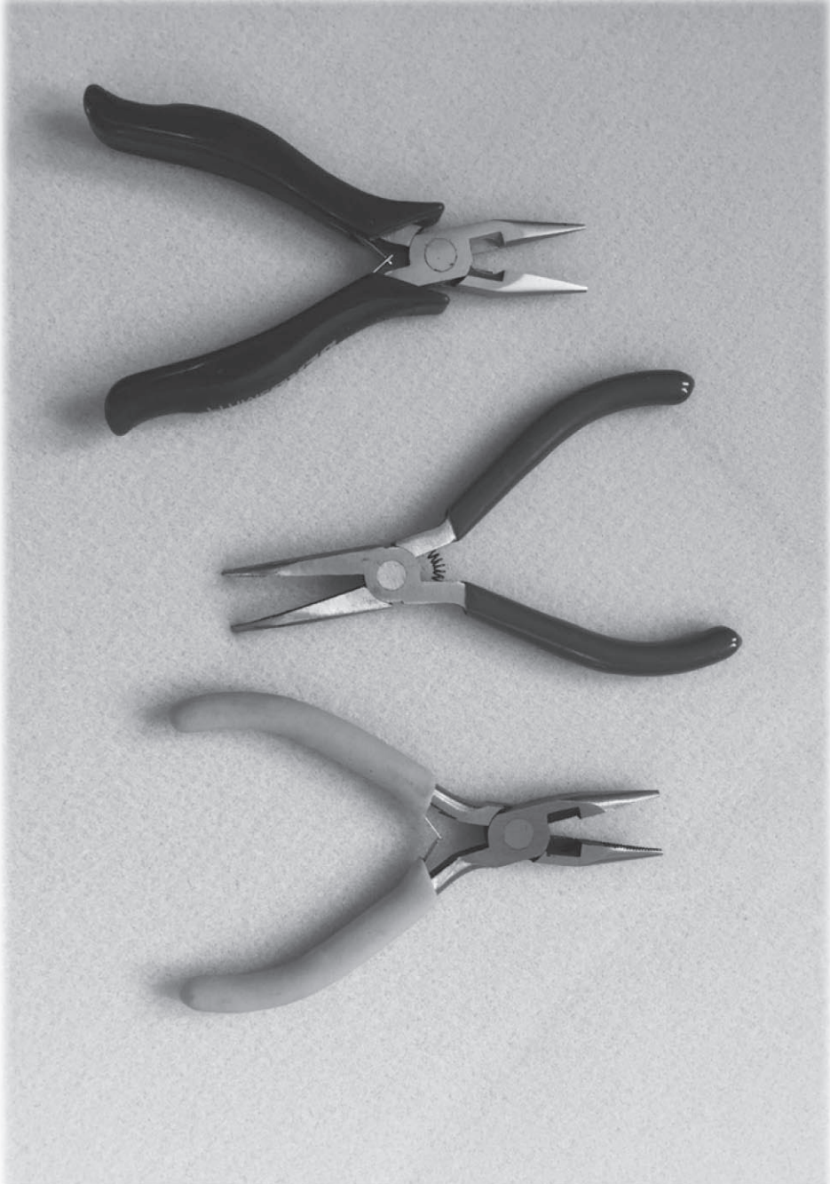
14. Jewellery pliers: top - flat nosed middle - bent nosed bottom - long nosed serrated jaws
